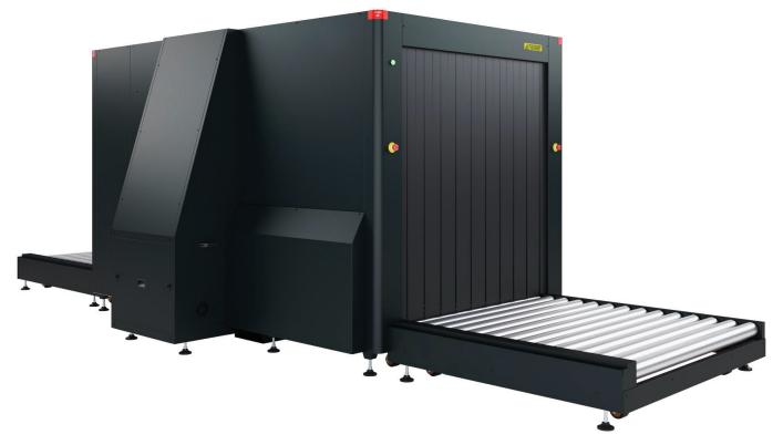
SecurSCAN XRC 150-165 is a large X-ray security system, specific for scanning pallets of goods and packaging, even very heavy ones. It allows the identification of organic and inorganic materials including counterfeit objects, contraband, weapons of all kinds, artisanal and conventional explosive devices (IED), liquid, solid, powdered drugs.
